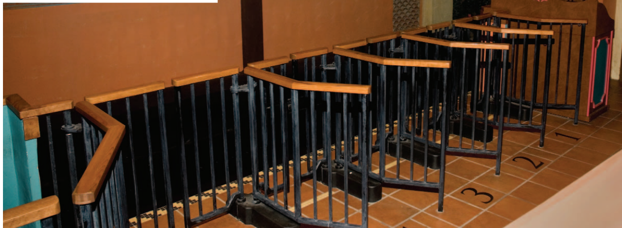
Secure station gates are designed to place a barrier between Guests in the ride-loading zone and the moving ride vehicle.
