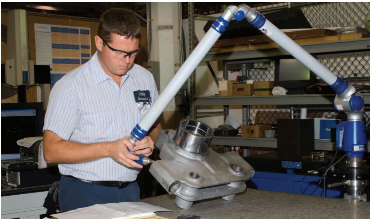
A Quality Assurance Inspector performs a dimensional inspection on a part.
